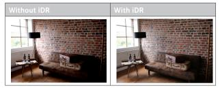
You can specify beforehand if and to what extent you want to optimize darker areas (High, Standard, Low, Off). In the Auto setting, the camera will automatically select the right setting depending on the contrast range of the object. In addition to that setting, the effect also depends on the exposure settings. The function will have the strongest effect in combination with low ISO values and fast shutter speeds. The effect is less pronounced with higher ISO values and/ or slower shutter speeds.
