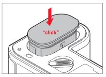
Insert the battery into the slot with the groove pointing towards the LCD panel and gently push until you hear and feel it clicking into place
