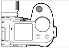
The shutter button works in two stages.
